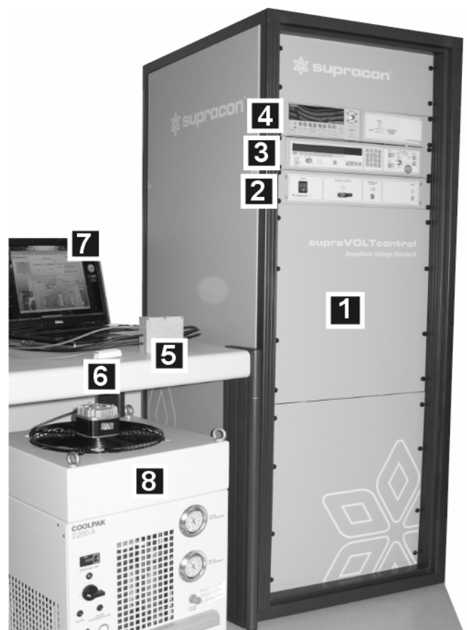
Fig. 1. Photograph of the cryocooler-based Josephson voltage standard system “supraVOLTcontrol” including the following components: 1: Pulse tube cooler with a SIS Josephson junction array and the 75 GHz microwave electronics installed in the 19” rack, 2: Control electronics, 3: EIP 578B source looking counter, 4: Keithley 2182A null detector, 5: 3-channel polarity reversal switch, 6: Sensors for temperature, pressure and humidity, 7: Laptop, 8: compressor unit with an input power of 2.5 kW.
