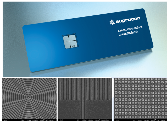
SEM-micrographs of the calibration pattern
